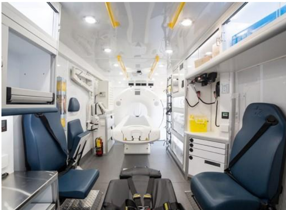
Figure 8: University of Tennessee Memphis Mobile Stroke Unit equipped with 16-slice Siemens Somatom Scope® scanner and head/neck CTA autoinjection system; with permission from University of Tennessee Health Science Center at Memphis, Mobile Stroke Unit
