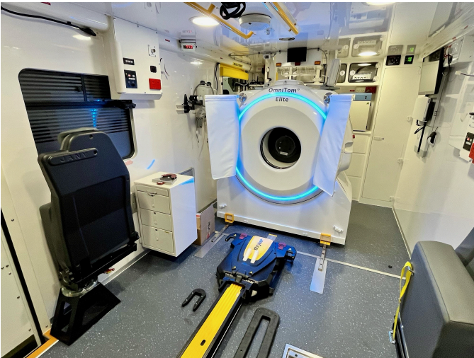
Figure 10. A view of the rear cabin of the Melbourne Mobile Stroke Unit, showing the OmniTom scanner, track for stretcher loading, and collapsed attendant seats. Reprinted with permission of The Melbourne Brain Centre at The Royal Melbourne Hospital.
